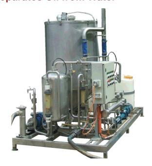
**IC-SEP -** This system works by separating the input waste by dissolving microscopic air bubbles (Dissolved Air Flotation) and floating one section of the waste stream up and out of the tank. This is the final stage that "polishes" the output stream removing residual traces of oil including emulsified and some dissolved constituents, prior to discharge to surface water.
