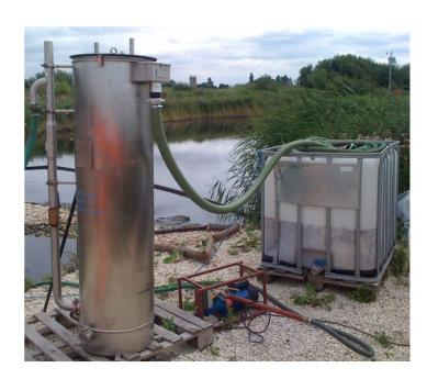
VGS - The Vertical Gravity Separator is a compact, cost effective unit developed to separate non-emulsified oil and water
